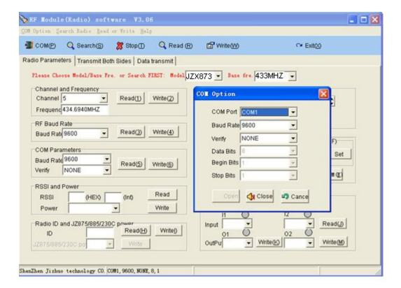
A, JZX873 module connected to the PC and plug in the power, select the serial port used.
