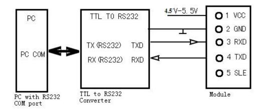
Note: As JZX873 mode TTL interface module, so the PC must be added to connect the TTL to RS232 converter, and converter must supply DC 5V of electricity.
