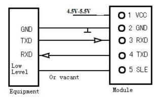
Note: JZX873 did not sleep in the state, the module of the SLE feet must be vacant. In the sleep state when the module must be low, the module can send and receive data.
