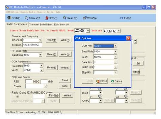
A, between the JZX861 module and connect a PC RS-232 to TTL adapter, and plug in the power, select the serial port used.
