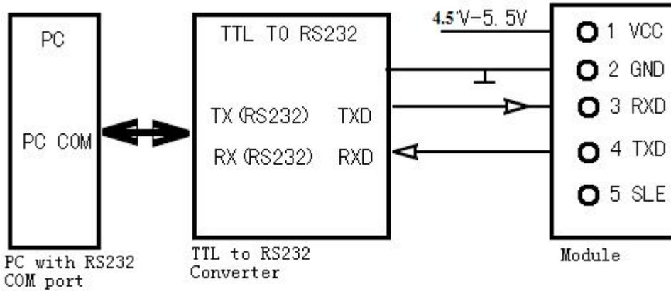
Note: As JZX874C mode TTL interface module, so the PC must be added to connect the TTL to RS232 converter, and converter must supply DC 5V of electricity.
