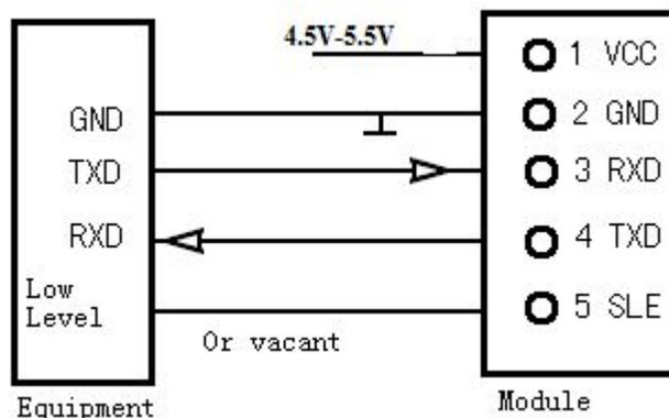
Note: JZX874C did not sleep in the state, the module of the SLE feet must be vacant. In the sleep state when the module must be low, the module can send and receive data.
